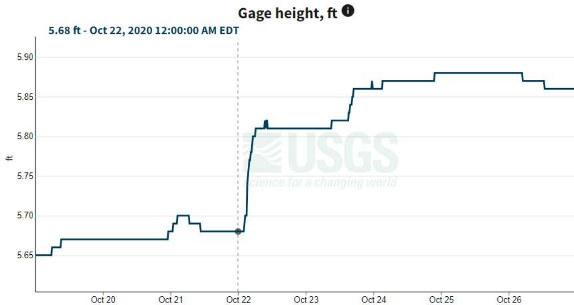
Figure 4: USGS Stream Gage Data for Pigeon Creek from October 19, 2020 to October 26, 2020 *Samples collected beginning at 10:15 AM on October 22, 2020
